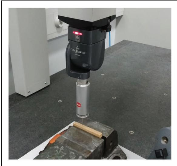
**Figure 7.** Scanning the surface in the coordinate measuring machine.
