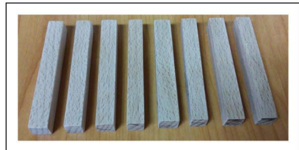
**Figure 3.** Photograph of samples with different depths of penetration during ball burnishing.
