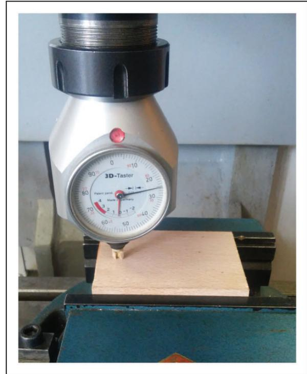
**Figure 2.** Photograph of control normality surface of the workpiece and the spindle axis vertical milling machine tool.
